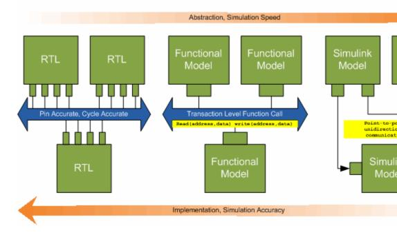
The functional model provides a sort of halfway point between the speed you can achieve with abstraction and the accuracy you get with implementation.
